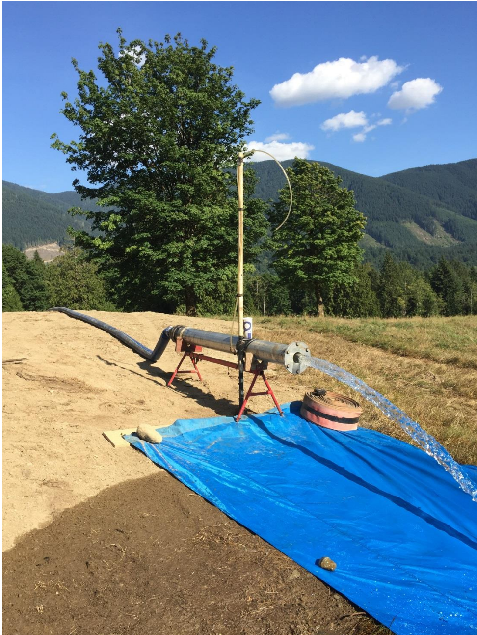
Photo 5: Water pumped from PW17-1 at a rate of 12.7 L/s during the constant rate test.
